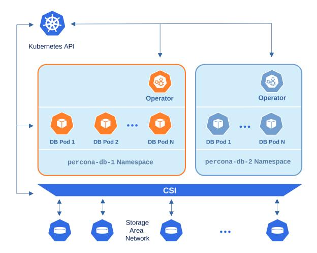
Normally this is a recommended approach, as isolation minimizes impact in case of various failure scenarios. This is the default configuration of our Operator.
