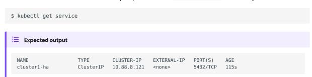
This service points to the active primary. In case of failover to the replica node, will change the endpoint automatically.
