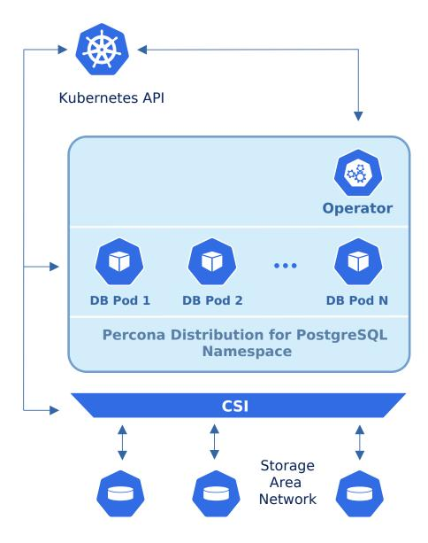
To provide data storage for stateful applications, Kubernetes uses Persistent Volumes. A *PersistentVolumeClaim* (PVC) is used to implement the automatic storage provisioning to pods. If a failure occurs, the Container Storage Interface (CSI) should be able to re-mount storage on a different node.
