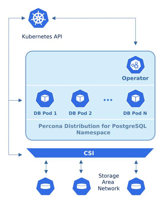
To provide data storage for stateful applications, Kubernetes uses Persistent Volumes. A *PersistentVolumeClaim* (PVC) is used to implement the automatic storage provisioning to pods. If a failure occurs, the Container Storage Interface (CSI) should be able to re-mount storage on a different node.
