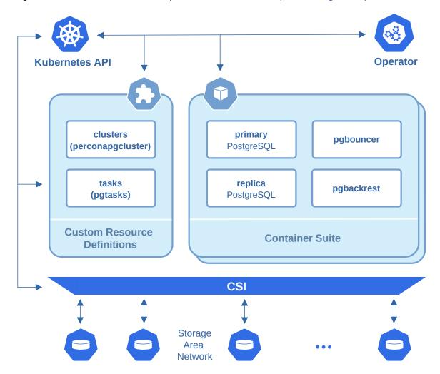
PostgreSQL containers deployed with the Operator include the following components:
