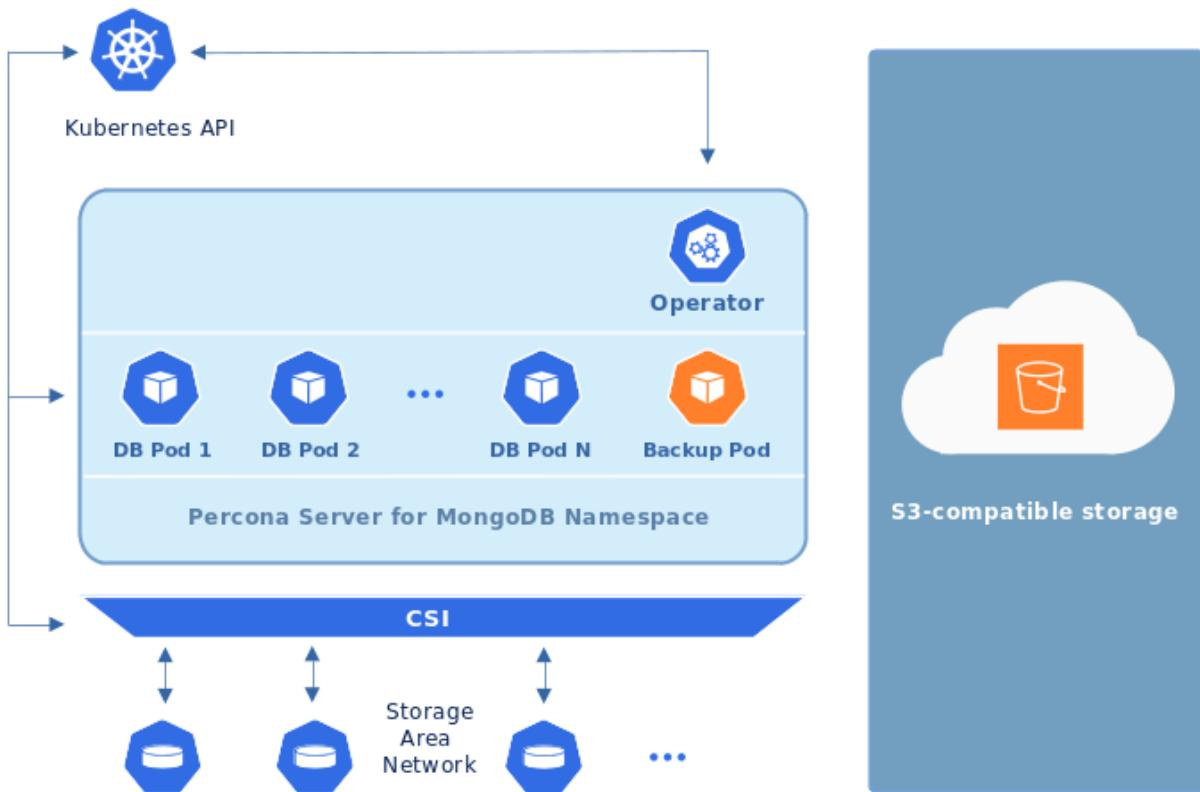
The Operator allows doing cluster backup in two ways. *Scheduled backups* are configured in the [deploy/cr.yaml](#) file to be executed automatically in proper time. *On-demand backups* can be done manually at any moment. Both ways use the [Percona Backup for MongoDB](#) tool.
