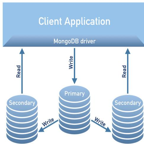
A replica set consists of one primary server and several secondary ones (two in the picture), and the client application accesses the servers via a driver.
