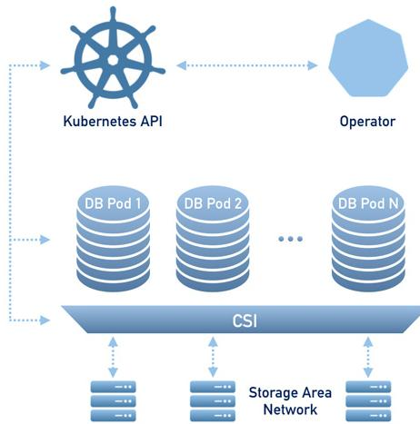
To provide data storage for stateful applications, Kubernetes uses Persistent Volumes. A *PersistentVolumeClaim* (PVC) is used to implement the automatic storage provisioning to pods. If a failure occurs, the Container Storage Interface (CSI) should be able to re-mount storage on a different node. The PVC StorageClass must support this feature (Kubernetes and OpenShift support this in versions 1.9 and 3.9 respectively).
