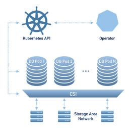
To provide data storage for stateful applications, Kubernetes uses Persistent Volumes. A *PersistentVolumeClaim* (PVC) is used to implement the automatic storage provisioning to pods. If a failure occurs, the Container Storage Interface (CSI) should be able to re-mount storage on a different node. The PVC StorageClass must support this feature (Kubernetes and OpenShift support this in versions 1.9 and 3.9 respectively).
